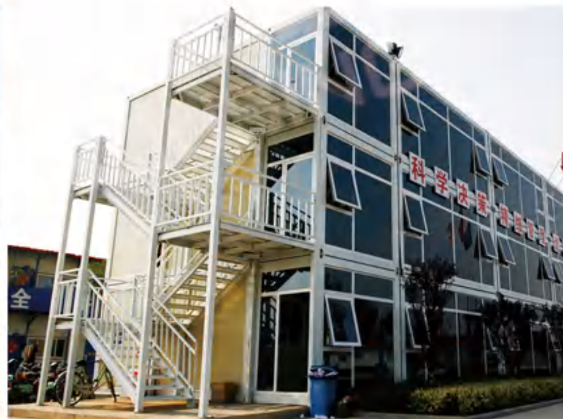
外置三跑楼梯 External three-run stairs
