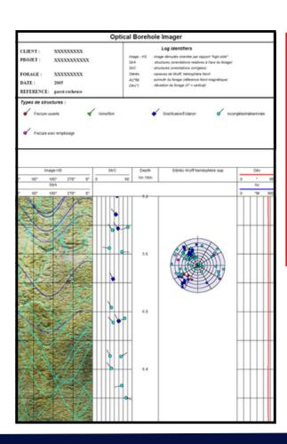
These data can be presented on the image logs themselves, or exported and used in other forms of analysis such as stereographic projections, rose diagrams of histogrammes. It is also possible to produce a synthetic RQD log based on the spacing between fractures observed on the image logs, these have shown to correlate well with observations made directly on the core samples.
