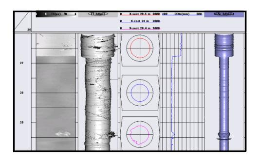
The principal application of this method lies in determining the local stress direction by analysing borehole ovalisation or breakouts.
