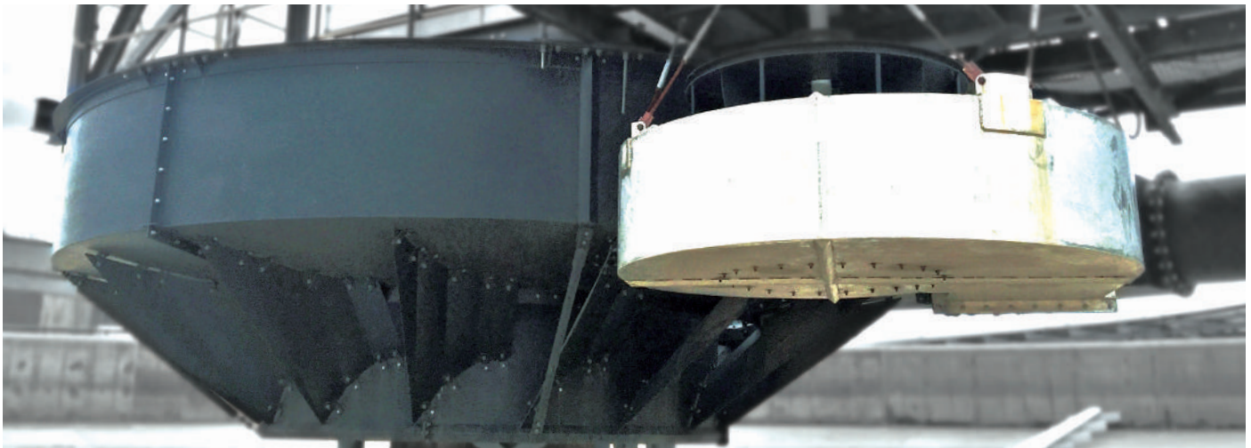
Above: Radflow™ feedwell (left) installed in a 50mØ thickener showing the ETAQ™ (right) dilution unit.
