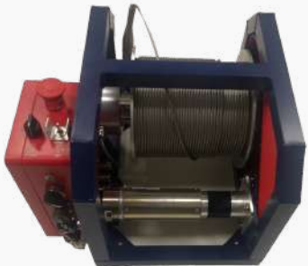
Borehole logging probes with datalogger and winches
