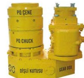
Nitrogen gas spring loaded jaws with hydraulic opening/spring closing function ensuring fail-safe operation.
