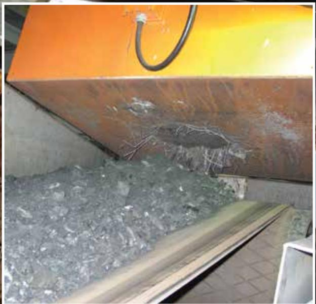
*Suspended magnets play an important role removing dangerous tramp or rogue metal from conveyed materials.*
