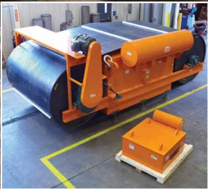
*For many years Eriez has provided oil-cooled electromagnets for heavy duty tramp iron separation applications. The parabolic shape of the field produced by these magnets makes them ideal for deep penetration of heavy burden depths conveyed on troughed belts or concentrated in a narrow flow.*
