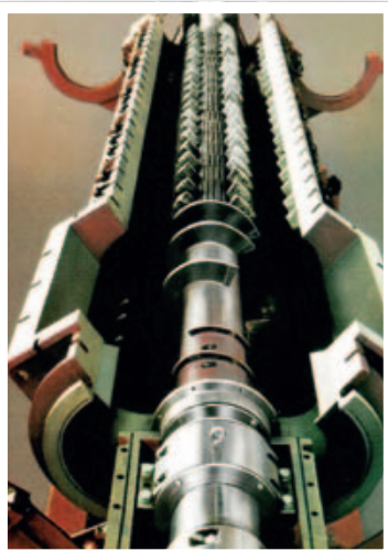
Complete continuous mixer/kneader with oscillating gearbox.
