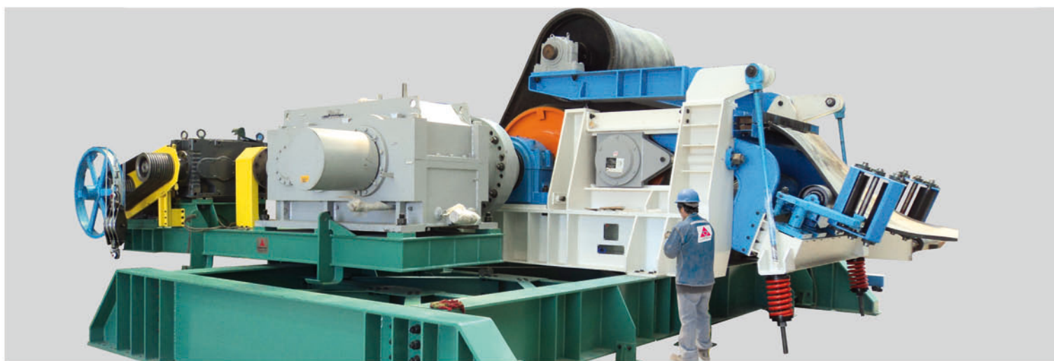
Temporary Drive Station
