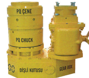
Nitrogen gas spring loaded jaws with hydraulic opening/spring closing function ensuring fail-safe operation.
