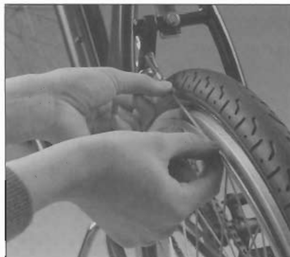
Figure 3: To inspect the brake band, loosen the band using the adjusting barrels shown above. Grasp the rim band with your fingers and pull it sideways out of the groove.
