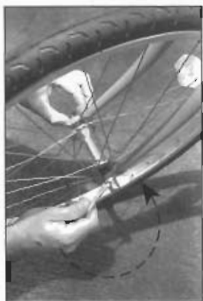
Figure 4: Once the quick-release mechanism is installed, install the front tire with the quick-release lever on the left side of the bike. Tighten the adjustment nut and flip the quick-release lever toward the rear of the bike. If the quick-release lever is too loose or too tight, release it and readjust the nut by 1/2 turns accordingly.
