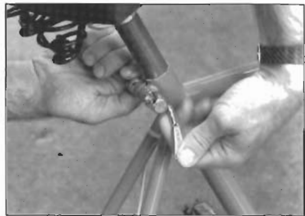
Figure 4: Loosen the seat quick-release lever and slide the seat into the seat tube. Tighten the quick-release lever when the seat is in the seat tube.
