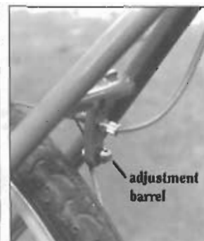
Figure 2: Another adjustment barrel is found on the frame by the rear wheel.
