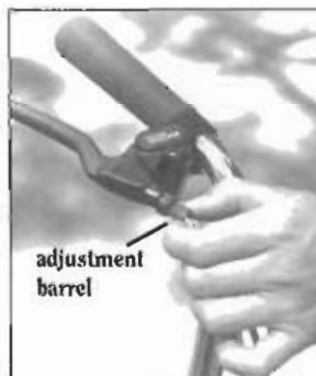
Figure 1: If the brake lever stroke becomes too long, the cable probably has stretched. To adjust the cable, turn the adjustment barrel found by the brake.
