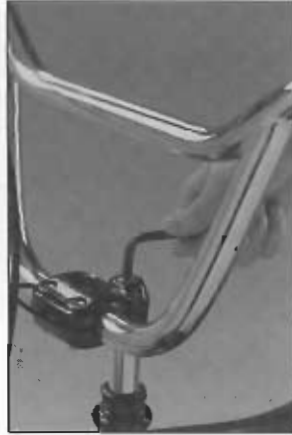
Figure 2: Position the handlebars and tighten the center bolt with the Allen wrench.
