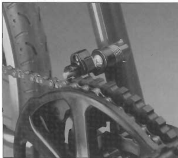
Figure 1: The gap between the cam brake pin and the cam plate teeth should be no less than 1/16 " as shown above.
