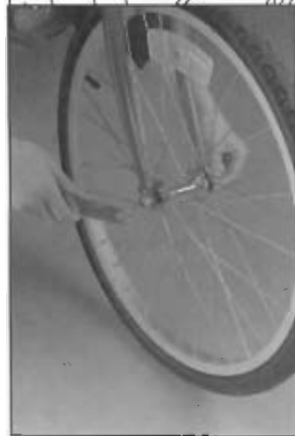
Figure 3: Slide the safety washers onto the axle bolt and insert the safety tabs into the slots above the axle. Place the nuts on either side of the wheel and tighten them with the flat wrench. •An arrow on the side of the tire indicates the tread direction. The arrow will point downward when you look at it from the riding position.
