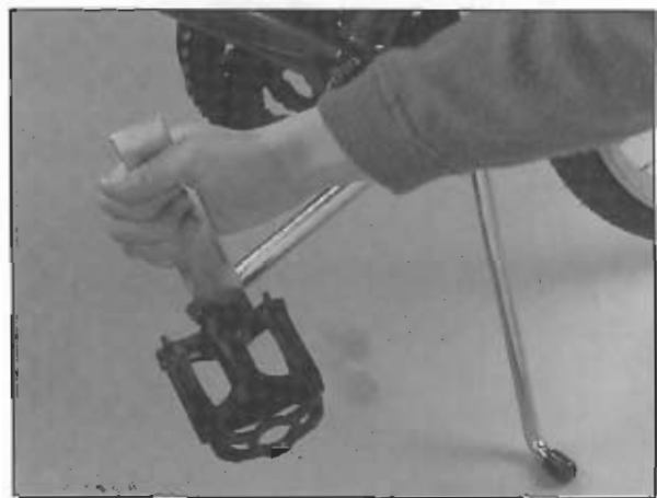
Figure 5: Attach the pedal to the crank arm with the flat wrench. The pedals are marked L or R on the end of the threaded stud for left and right side.
