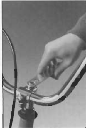
Figure 2: Position the handlebars and tighten the center bolt with the flat wrench.
