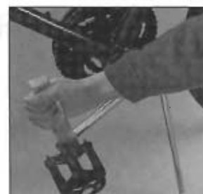
Figure 6: Attach the pedal to the crank arm with the flat wrench. The pedals are marked L or R on the end of the threaded stud for left and right side.
