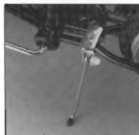
Figure 7: Insert the bolt through the lock washer and top plate. Place the bolt assembly in position as shown above. Tighten the bolt with a 9/16" wrench or provided flat wrench.
