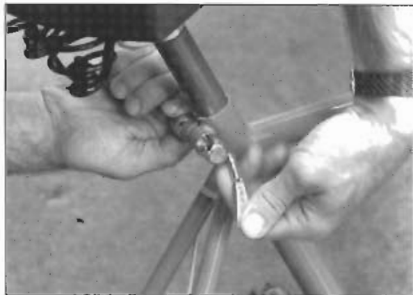
Figure 5: Loosen the seat quick-release lever and slide the seat into the seat tube. Tighten the quick-release lever.
