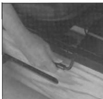
Figure 6: Pull up on the bar beneath the seat to adjust the seat position.
