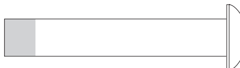
Boulon de Renforcement 3/8" x 2 1/4" (31)–2
