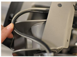
FREE CABLE IN LOOP SHOULD BE APPROXIMATELY THIS LENGTH.
