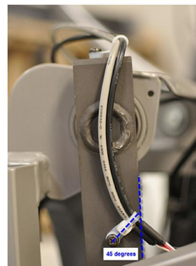
RIGHT ROCKER SHOWN. ROUTE CABLE WITH 101416-001 AS SHOWN. BOTTOM CABLE TIE TO BE ALIGNED AT 45 DEGREES TO EDGE OF ROCKER.
