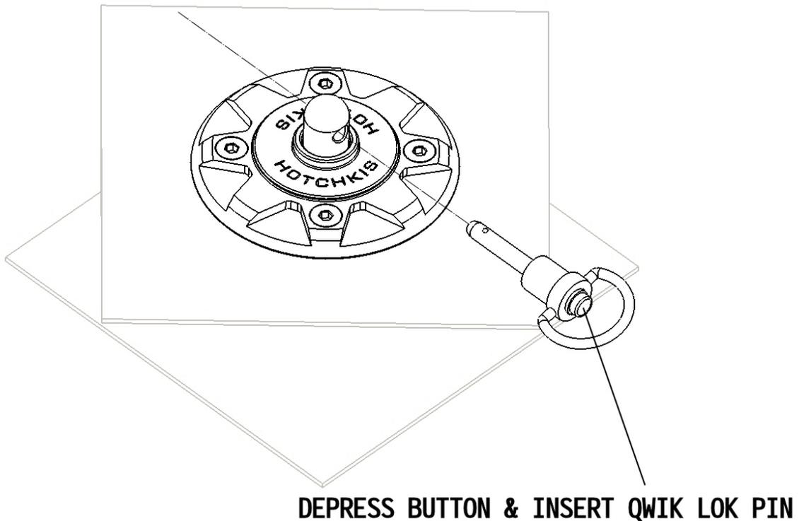
If the Qwik Lok clip does not sit snugly onto the hood base when the hood is closed and shows a gap, then you will have to loosen the pin nuts and lower the pin.
