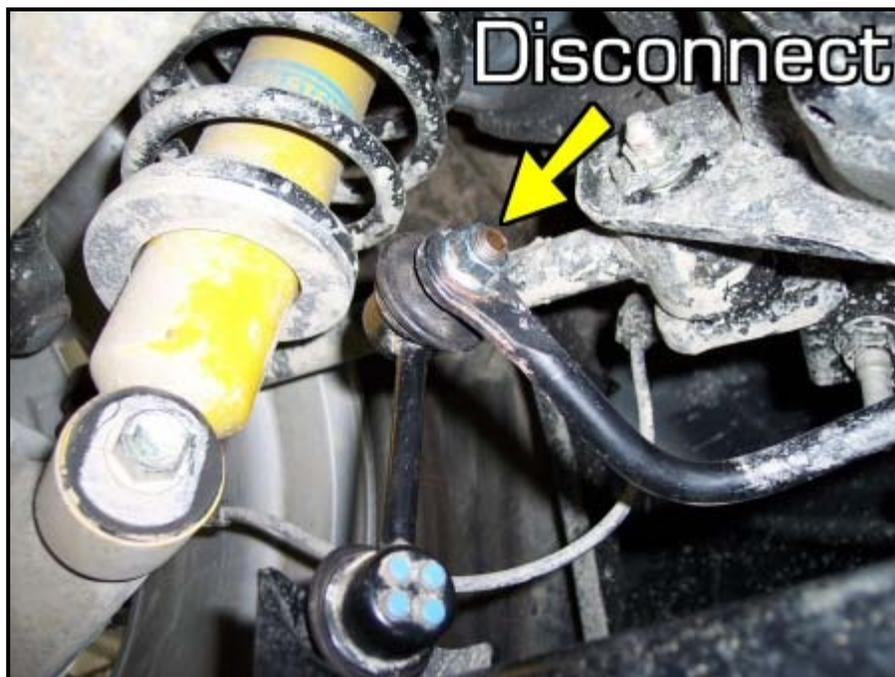
3R *Undo the Sway Bar Bushing Bracket Bolts*
