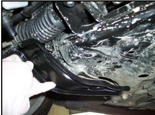
5F *Undo the Sway Bar Bushing Bracket Bolts*
