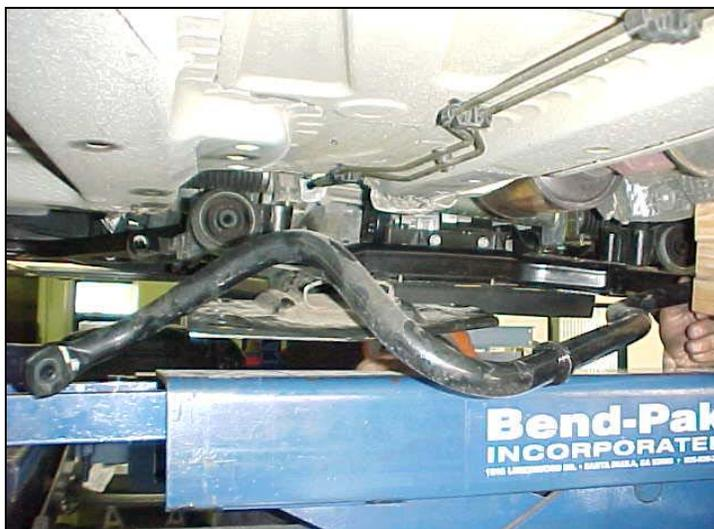
9/ **Before installing the bushings or brackets**, install the HSport bar the same way in which you removed the stock bar. The center HSport sticker faces right-side up and to the rear of the vehicle.
