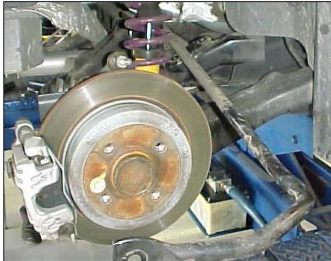
8/ Once the stock bar is out, slide the Hotchkis bar in without the bushings and brackets attached. Once the bar is in the approximate stock location, use the remaining grease on the inside of the rear bushings and slip them over the bar. Then install the supplied bushing brackets with the grease fittings pointing to the outside.
