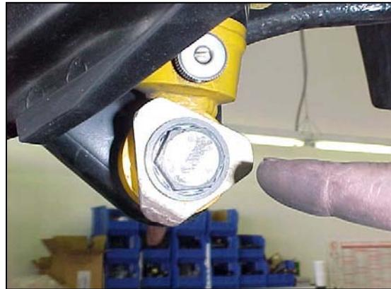
5/ Before removing the sub-frame hardware, remove the four anti roll bar bushing bracket bolts using a 13mm wrench or socket.
