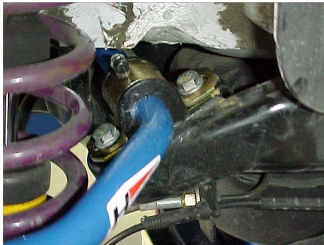
9/ Now, reinstall the 4 sub-frame bolts, bushing bracket bolts, spring/shock assemblies and end-links. Start the end links in the middle position and tune from there. Make sure all hardware is secure and tight.
