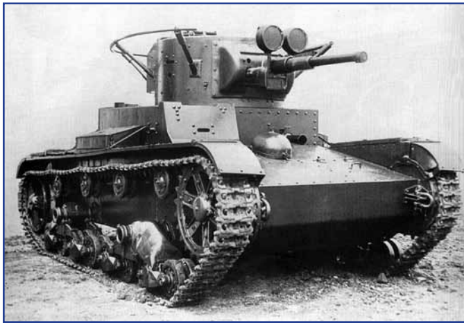
The T-26 m33 tank with the rail antennae and turret spot-lights.
