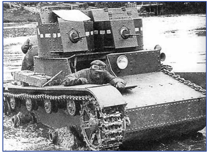
Produced in large numbers, the Soviet T-26 m31 tank was armed with twin machine guns in independent turrets.
