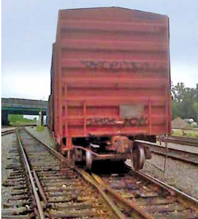
Parking a railcar too near a switch causes clearance problems for trains passing on the adjoining track.
