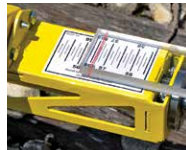
Gauge scale (55.5 - 58.5") can be read through a lexan lens from either side of Roadmaster.
