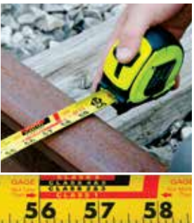
Measure Track Gauge
