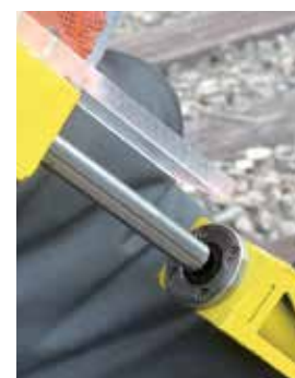
Two-piece assembly features spring-loaded piston for precise gauging.
