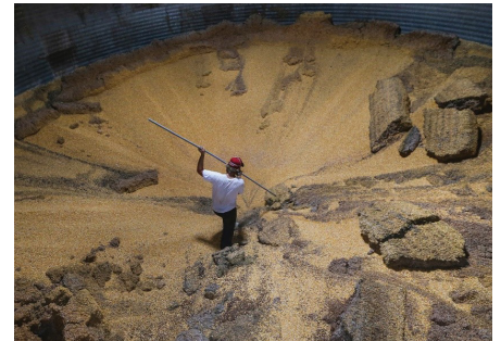
Rodding grain to unplug the sump while equipment is running is the #1 cause of grain engulfments.
