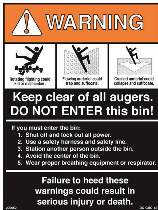
Figure 10: Safety decal for grain bin access
