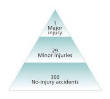
Safety Pyramid Developed by H. W. Heinrich (1931)
