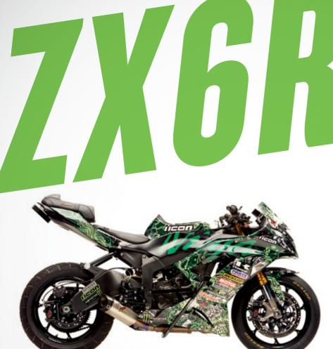
Modern freestyle bikes use a reshaped passenger seat with a large opening for foot placement. The passenger pegs are then replaced with a reinforced subcage. Low-profile crash cages and tucked subframe grind plate minimize damage when the bike is dropped, and the bike is always dropped. While the motor is left primarily stock, electronics are relocated or bypassed. This allows a stuntbike to run regardless of the myriad of
