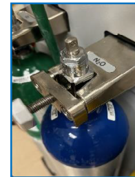
Integrated N 2 O E-cylinder attachment.
