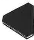
Cut a cardboard triangle with sides the length of the spacing you want.
