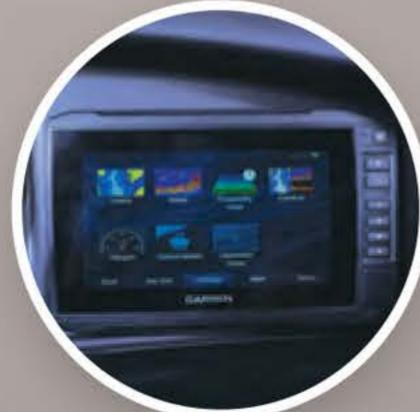
Garmin GPSMAP® 742xs 7" Touchscreen ClearVü GPS with Traditional CHIRP Sonar
