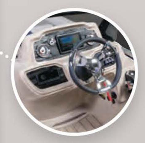
Tilt steering, Bluetooth stereo, motor gauges, 7" touchscreen Garmin Echomap GPS/ Fishfinder.
