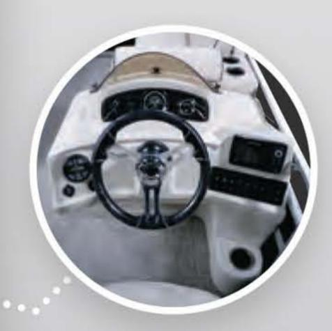
Fibreglass console has a Bluetooth stereo, Helix 5 GPS fishfinder, illuminated gauges and switches, and a deluxe steering wheel with tilt steering.
