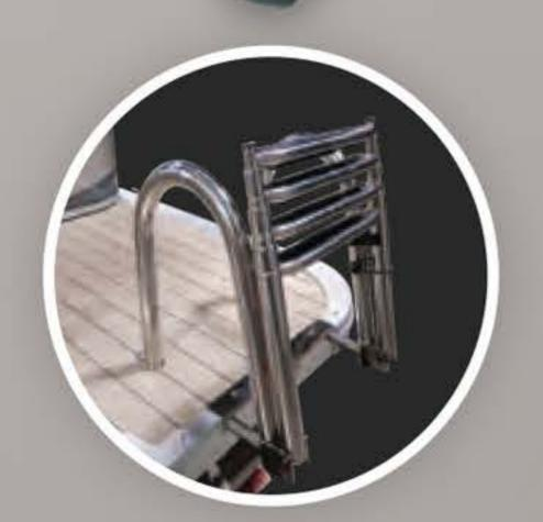
Large aluminum boarding ladder makes it easy to climb aboard from a dip in the lake.
