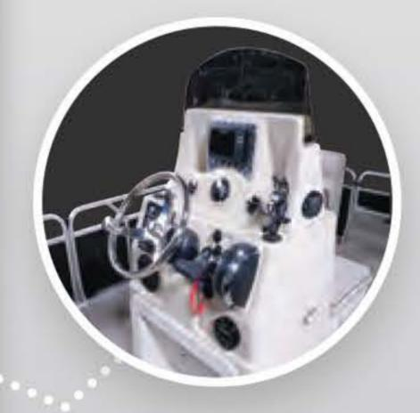
Fibreglass console with built-in Helix 5 GPS fishfinder, bluetooth stereo, illuminated gauges and switches, stainless steering wheel and MP3 port.
