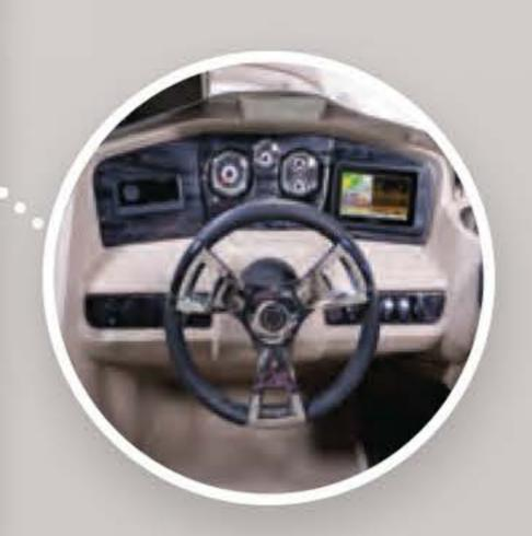
Tilt steering, Bluetooth stereo, motor gauges and 7" Garmin Touchscreen Echomap GPS.
