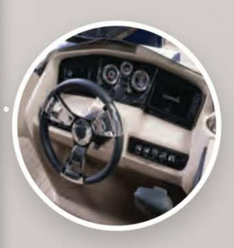
Tilt steering, Bluetooth stereo, motor gauges and 7" Garmin Touchscreen Echomap GPS.
