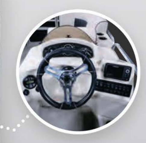
Fibreglass console has a Bluetooth stereo, Helix 5 GPS fishfinder, illuminated gauges and switches, and a deluxe steering wheel.
