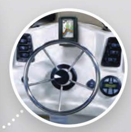
Fibreglass helm has a PiranhaMax4 fish/depth finder, Bluetooth stereo and stainless steel ship's wheel.
