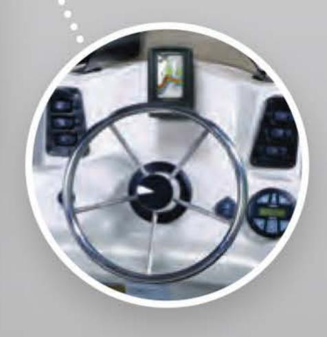
Fibreglass helm has a PiranhaMax4 fish/depth finder, Bluetooth stereo and stainless steel ship's wheel.
