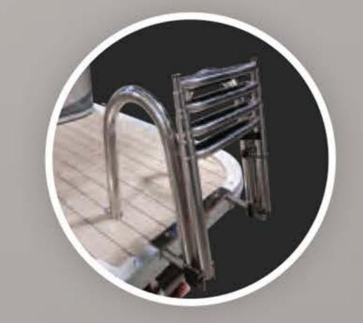
Large aluminum boarding ladder makes it easy to climb aboard from a dip in the lake.
