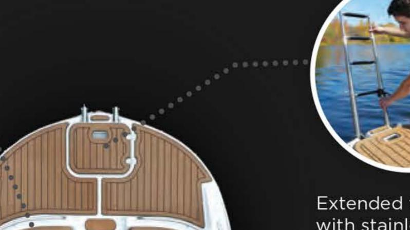
Extended front deck with stainless steel retractable bow ladder and non-skid mats
