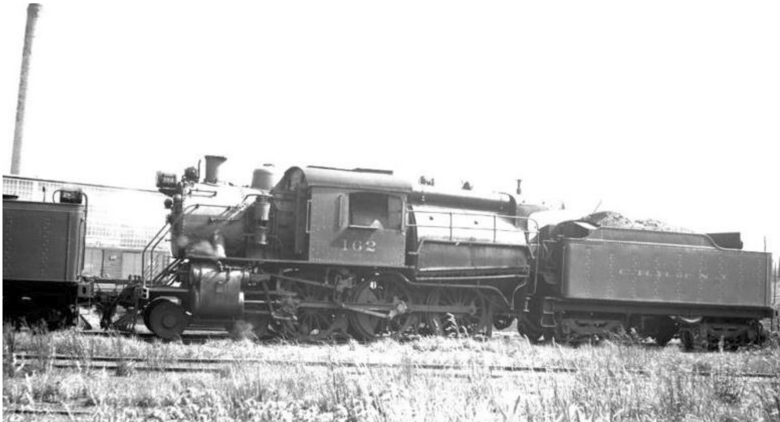
A CNJ Camelback Locomotive: Designed to burn anthracite coal, it's firebox was too wide to provide for adequate visibility
