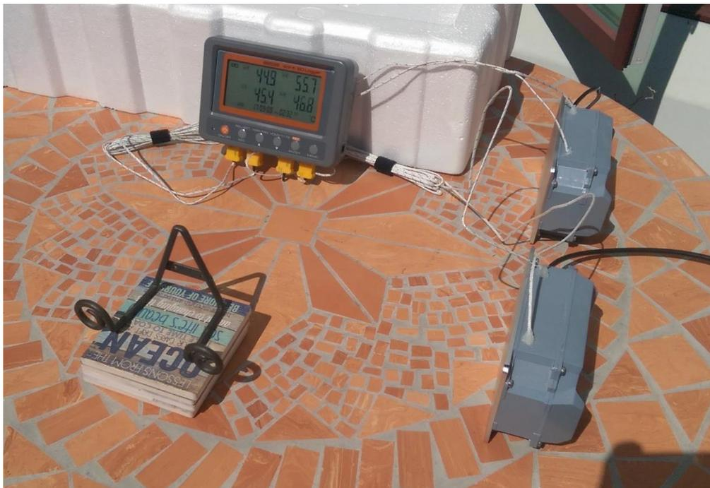
(data logger top row no heat sink: plate temperature, internal air temperature; bottom row heatsink: plate temperature, internal air temperature)
