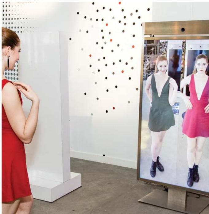
Figure 1: Customers can see a 360-degree view of themselves or view two images on a split screen.
