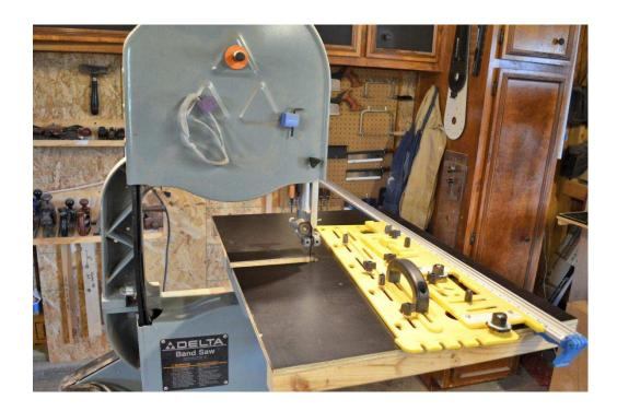
Some form of elaborate fence system could be used here, but the simple clamping straight edge that Scott showed us is quick, easy and reliable. It also allows for setting an angle to account for blade 'drift' if needed.
