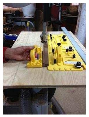
Scott had added a simple plywood extension table onto his 14" bandsaw and used a clamping straight edge as the fence. Brilliant!
