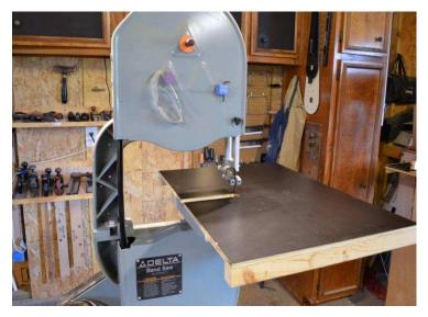
A leftover side from a shipping crate was the basis of this table. The ply was a bit rough, so it was sanded and laminated to provide a smooth working surface.
