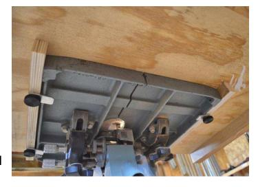
bandsaw table and are tightened to it with the knobs. Fender washers would work great, if you have some on hand.
