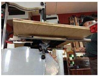
Scott's band saw has a pair of steel tubes already mounted so he used toggle clamps to connect his table onto the saw.
