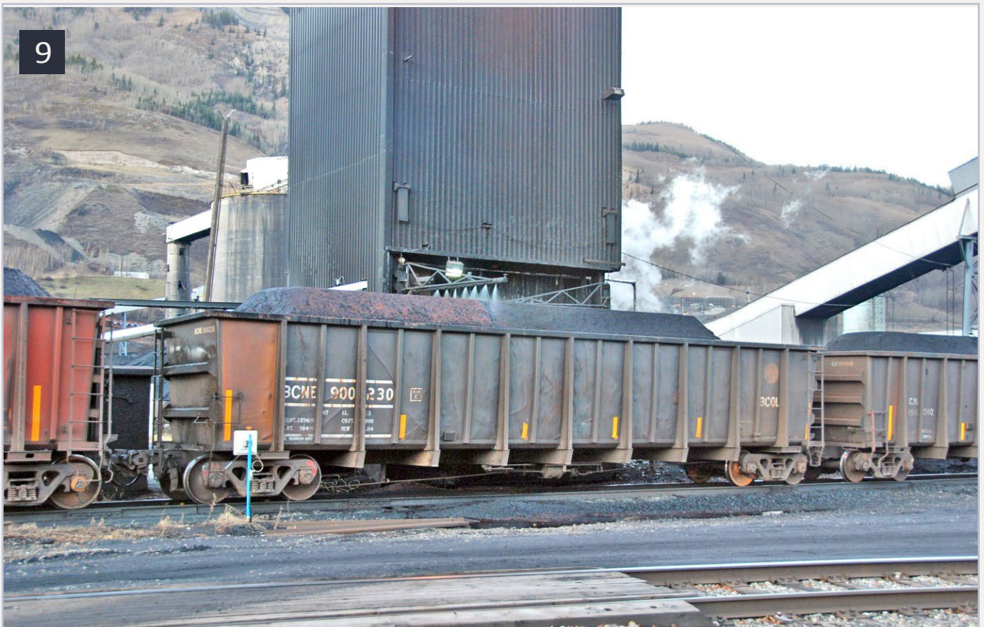
9. Coal load being sprayed with latex to reduce dust.
