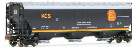
**ScaleTrains.com** has released an N scale version of a Gunderson 5188 cu. ft. triple-bay covered hopper car. The ready-to-run model features photo-etched stainless steel see-through roof walk and end platforms, metal grab irons, plastic semi-scale Type E lower knuckle couplers, uncoupling levers, trainline hoses, and ASF Ride Control trucks.
