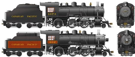
For Canadian Pacific modelers, Rapido will offer a D10 Class 4-6-0 Ten Wheeler. CPR's D10 was the most numerous class of steam locomotive in Canada with 502 being built between 1905 and 1913. Many lasted until the end of steam service in 1961.
