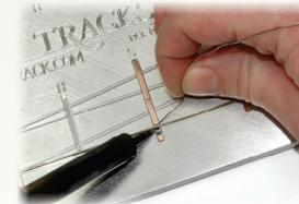
The Fast Tracks PointForm tool makes it fast and easy to file perfect frog and switch points for the turnout.
