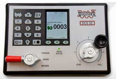
**Digitrax** displayed a wide range of electronic items in their Amherst booth including their DCS 52 Zephyr Express, a 3.0 amp Loconet command station, booster, and throttle. This latest version features a backlit 3D
