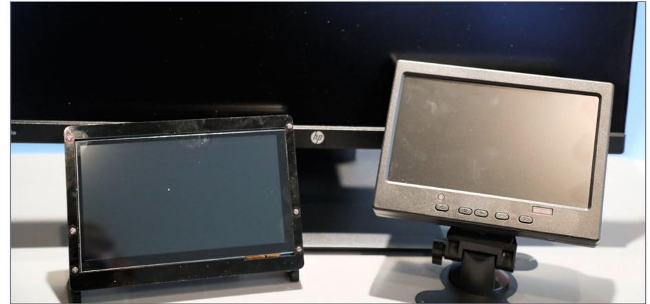
8. Displays with HDMI Interface (24-Inch & two 7-inch).
