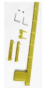
Moloco sells an HO scale version of a Morton metal roofwalk for a 50-foot car. The edges on the etched parts are pre-fold, just like the prototype. The kit includes a high brake wheel platform and two bottom crossover walkways suitable for cushioned cars. One of the walkways has a cutout for the brake linkage. A pair of corner grab irons and eyebolts are included. For additional information visit [www.molocotrains.com](http://www.molocotrains.com).
