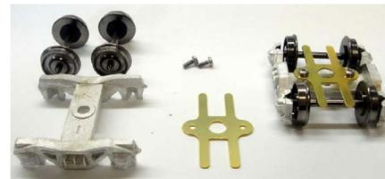
After mentioning Bowser's new tender trucks last month we later obtained photos to illustrate the new items. The four-wheel Kiesel rigid tender trucks include a one-piece cast frame with 36-inch wheels and a brass retainer.
