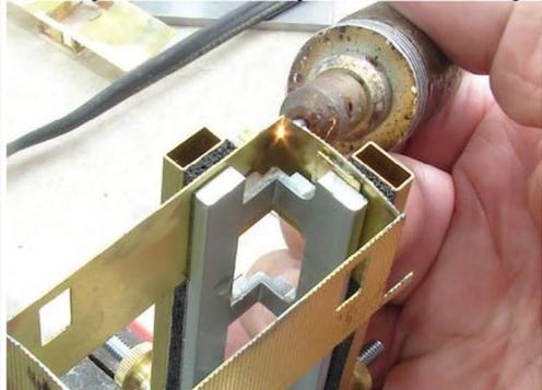
Clamps for soldering and gluing!
