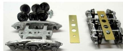
The kit for the six-wheel Buckeye tender truck also comes with 36-inch wheels. The retainer plate has two center clearance holes that allow optional positions for the truck's bolster mounting. For additional information contact a dealer or visit [bowser-trains.com](http://bowser-trains.com).
