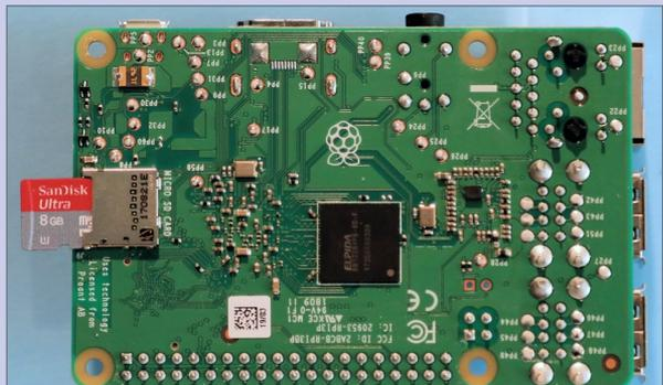
**11. Micro SD memory card inserted into RPi socket.**
