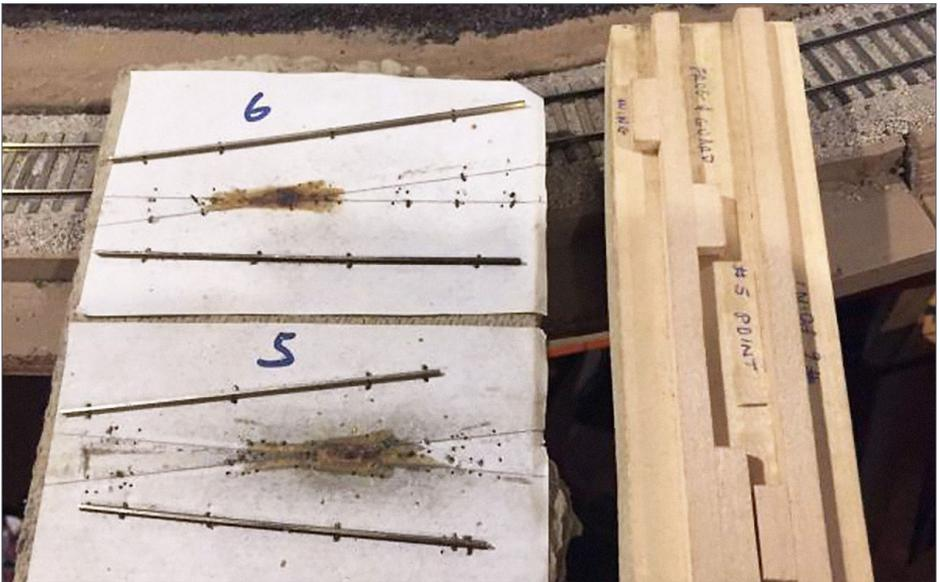
3. Jigs for cutting rail allow all pieces to be cut to the same length and create a "kit" of prefabricated pieces.
