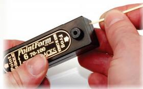
Just insert the rail into the tool and file.
