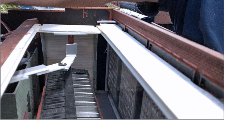
11. The linkage arms and attachment to the underside of the door. You can see some of the patchwork linkage arms where adjustments were made for smooth operation.
