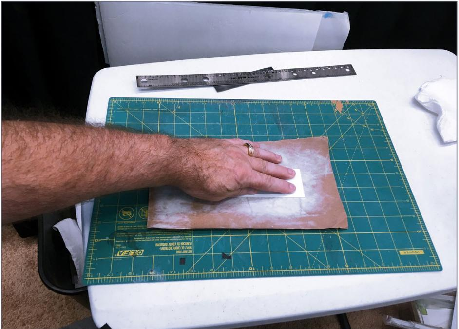
6. The door material needs to be sanded extra-thin to flex through the curving door track channel.
