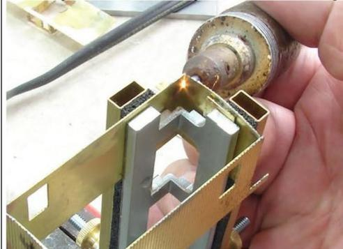
Clamps for soldering and gluing!
