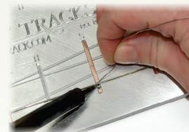
The Fast Tracks PointForm tool makes it fast and easy to file perfect frog and switch points for the turnout.
