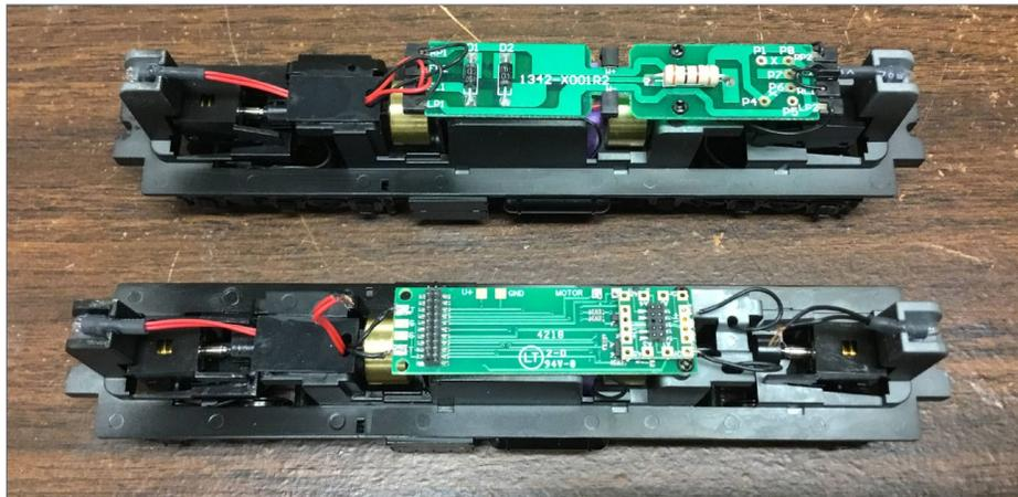
10. Two of Jim Moe's Proto1000 RSC2s before (top) and after (bottom) installing the Decoder Buddy. Sugar cube speakers might now fit in the extra space.
