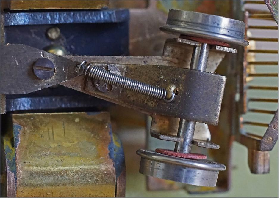
2. Some engines have a coil spring attached to the frame (left) and to the pilot truck (right). A longer spring will reduce down-force and a shorter spring increases it. Other engines will have a coil spring placed vertically to exert pressure. Clipping off one coil could increase pressure. Adding a spacer or stretching the spring will decrease pressure.
