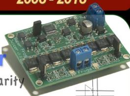
Automatic DCC Polarity Reverser
