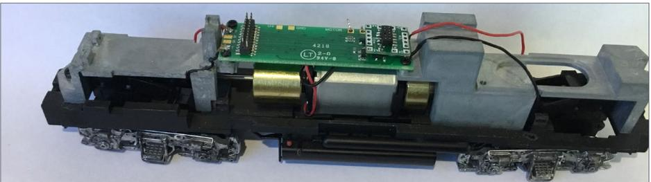
7. This is a new Atlas Silver DC decoder replacement. The Decoder Buddy installs in both directions and screws-in directly. In this locomotive the connector board should be accessible through the hatch on top.
