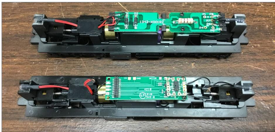
10. Two of Jim Moe's Proto1000 RSC2s before (top) and after (bottom) installing the Decoder Buddy. Sugar cube speakers might now fit in the extra space.
