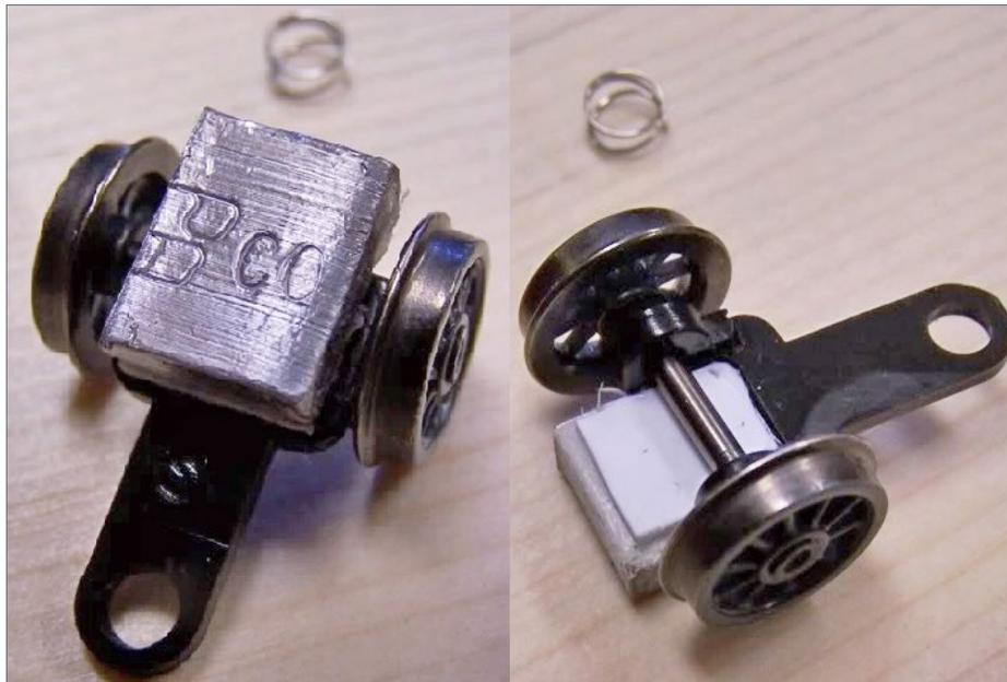
1. HVT Dave chose not to reduce weight on the drivers of his engine, so he removed the pilot truck spring, then added a weight directly to this Bachmann 2-6-0 pilot truck. The changes solved his derailment issues instantly. The top view (left) and bottom view (right) show the automotive stick-on wheel weight. *HVT Dave photo*
