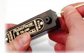
Just insert the rail into the tool and file.
