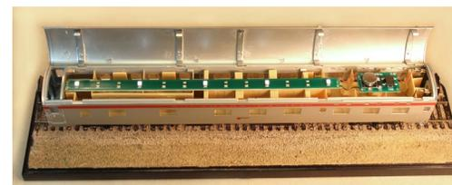
SP Daylight/Limited Editions has released a DCC/DC constant lighting kit for use in Walthers HO scale lightweight passenger cars. The kit is composed of two PCB peel 'n stick boards, wiring, and connector
