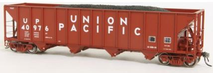
Tangent Scale Models is selling several versions of an N scale Bethlehem 100-ton 3600 cu. ft. quad-bay open hopper cars. The models are based on a
