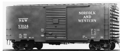
**Kadee** has scheduled the release of a Norfolk & Western 40-foot PS-1 boxcar next month. The HO scale ready-to-run model closely follows prototype car No. 53124 built by Pullman Standard in 1953. Both the model and the full-size boxcar were fitted with 8-foot Youngstown sliding doors.
