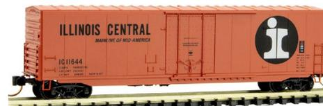
Micro-Trains N scale version of this IC 50-foot steel box car has an 8-foot plug door. The model represents a prototype
