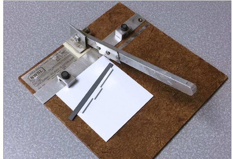
8. The stripwood to be cut is placed on the back side of the fence for the first cut.
