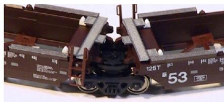
The cars are equipped with Kato's Kinematic trucks that remain closely coupled on straight track and flex for smooth operation on curved track. For additional information contact a dealer or
