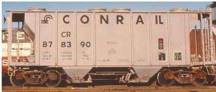
Kadee's June production schedule includes an HO scale version of Conrail's No. 878390 PS-2 twin-bay covered hopper. The prototype was built in 1956 and repainted with light gray
