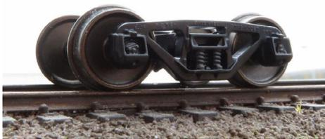
Depending on the road name being modeled, some of the gondolas will be fitted with Rapido's 70-ton trucks that have roller bearings retrofitted into the journal boxes.
