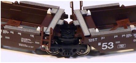
The cars are equipped with Kato's Kinematic trucks that remain closely coupled on straight track and flex for smooth operation on curved track. For additional information contact a dealer or
