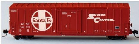
**Wheels of Time** has scheduled a second run of its N scale Pacific Car & Foundry 50-foot 70-ton exterior post insulated boxcars. They are expected this
