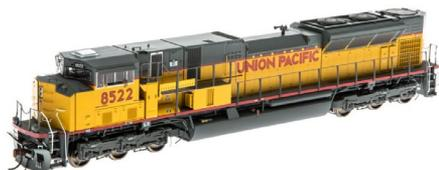
Features unique to the Union Pacific version will include an antenna dome on cab roof, no window in the nose door, and extended sun shades on the cab windows.
