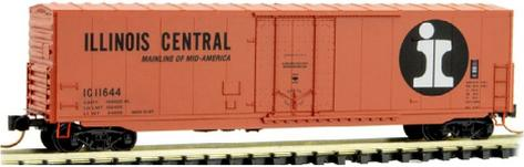
Micro-Trains N scale version of this IC 50-foot steel box car has an 8-foot plug door. The model represents a prototype
