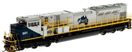
modifications to the former Union Pacific locomotive to meet Australian standards include the addition of a safety rail in the middle of handrails, FMG electrical junction boxes on the pilot, and special dual train line air hoses.
