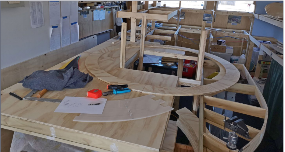
13. Fitting the helix on to the tabletop.
