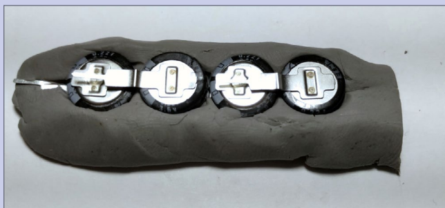
9. Caps in clay "jig" awaiting solder, with side B up.
