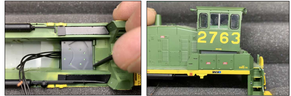
40, 41. Using the flat-blade screwdriver, release the last two locking lugs to finish releasing the cab.
