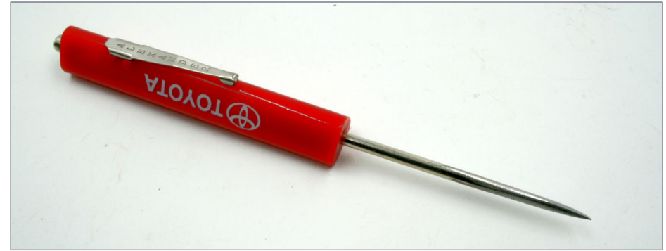
31. Grinding down the end of an inexpensive small screwdriver to a point makes a handy uncoupling tool. I glued a small rare-earth magnet on the handle to activate a caboose sound car decoder for coupling/uncoupling.
