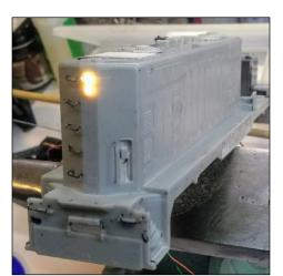
19. I spaced the LEDs on the PCB tie so they lined-up perfectly with the locomotive's headlight lenses. The PCB tie made for easy mounting to the locomotive shell.
