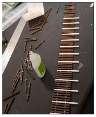
3. With every fifth tie removed. I added longer bridge timbers to support the deck and walkway.
