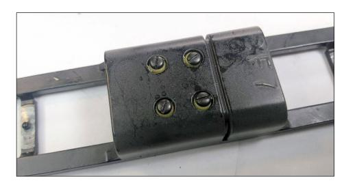
4. Test fitting the screws to the frame.
