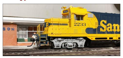
11. Santa Fe 2233 is an Athearn Genesis model of a GP7u. Except for an upgrade to LEDs, this unit is as it came from the factory, with Tsunami sound. The rotary beacon has a flash pattern that mimics the brightness of a Stratolite, but without any real rotation.
