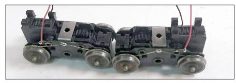
9. I added phosphor bronze wires to serve as wheel wipers to help provide more reliable power pickup and soldered feed wires to the truck frames.
