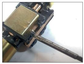
5. I tapped holes in the motor cradle to accommodate mounting screws.
