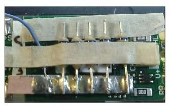
27. The PCB board with the resistors and blue function common wire attached. The anode wires from each LED function will attach to the other ends of the resistors. Note that the resistor leads are trimmed flush to the PC board on the one side and to about 1/8" on the other.
