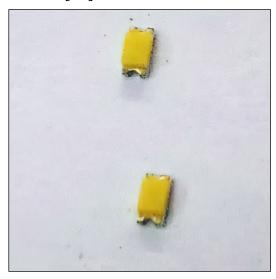
For the rest of the project, I used 0603 SMD LEDs, which have the advantage of being able to fit just about anywhere [15]. You can purchase 0603 LEDs already wired, but I like to solder my own wires to them. I prepare the LED
