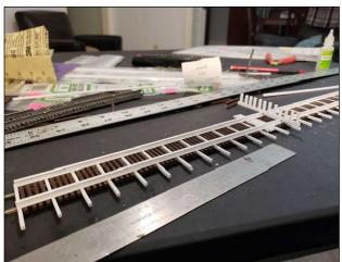
4. I used 3/8" styrene I-beams for the bridge's girders.
