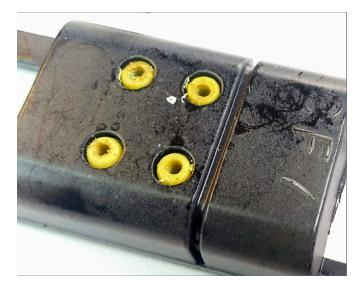
2. I drilled no. 43 holes through the rubber mounting lugs to accommodate screws.
