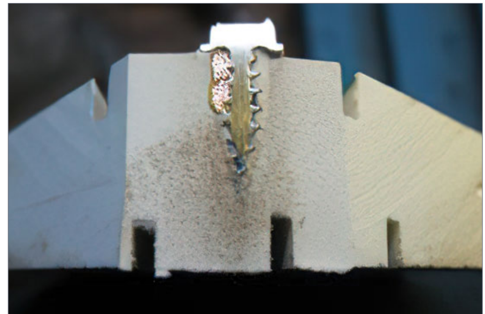
3. Cross-section through wires and the screw.
