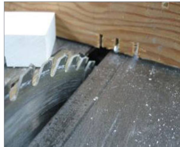
12. Screw is \frac{1}{2} " from blade for spacing grooves.
