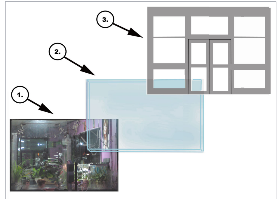
21. To make modern aluminum vestibules, begin with a photo of a lobby or entry scaled to size and printed (1). Overlay it with a 1/8"-thick piece of clear acrylic, cut to size (2). Cut a frame from silver wrapping paper, and position it on the acrylic (3). Use a toothpick to apply DAP Weldwood or similar adhesive around the edges.
