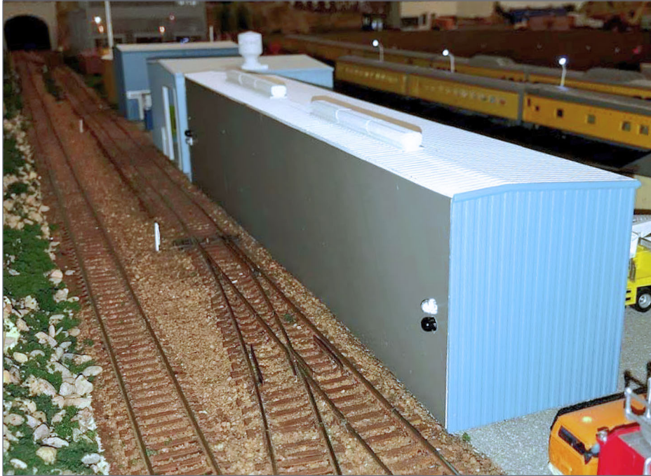
9. The infrared sensors shine a beam across the track to detect trains, which reflect it back to the sensors.
