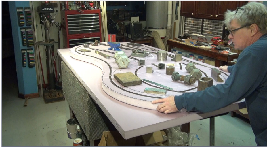
11. Ken then uses a variety of weights to ensure that the Great Stuff Pro will not force the foam layers apart.
