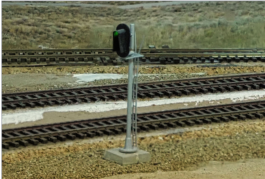
4. We chose a D-type signal with three LEDs and a snow hood.
