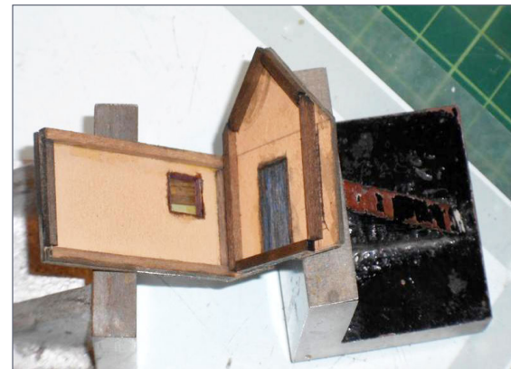
14. 8x8 timbers formed the bracing. Note the inset on the sides of the end wall to maintain fit with the side walls.
