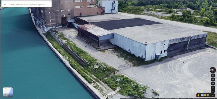
11. There were no tell-tale signs of tracks to the north of the loading bays. The concrete apron and truck wheel marks on the gravel lot to the right suggest this is a truck loading/unloading area.
