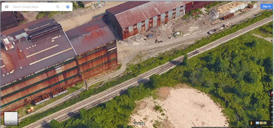
19. This lower-angle Globe View screen capture of the melt shop shows the weathering of this and other buildings, roof details, and additional details such as the ingots in gondolas spotted alongside the furnace.
