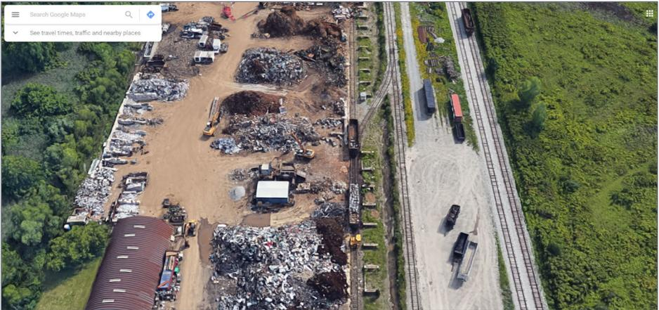
22. The scrap yard, just north of the furnace building, seen from the north. Notice the arrangement of tracks with scrap hoppers, the sorted piles of scrap, and the parking area for trucks.
