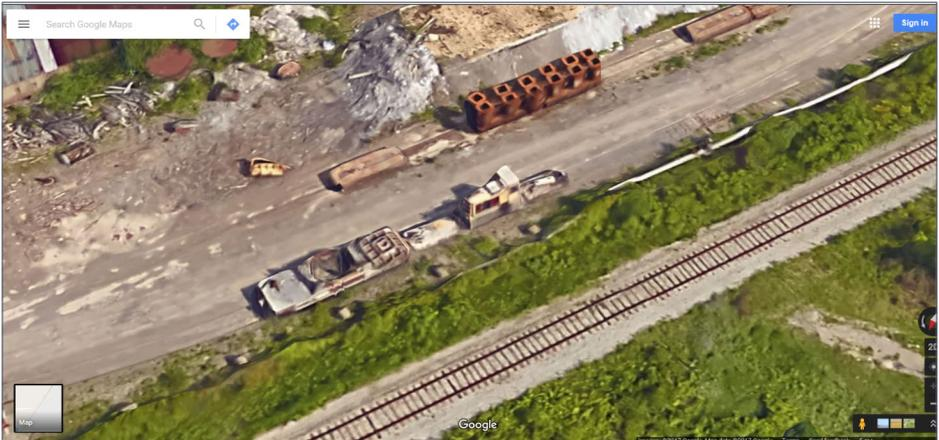
20. This zoomed photo of the far-right portion of [19] reveals a plant industrial switcher with idler cars and another piece of Valbruna ASW rolling stock on the siding south of the carbon electrode melt shop. On a track beside the switcher, ingot molds sit on another mill rail car.
